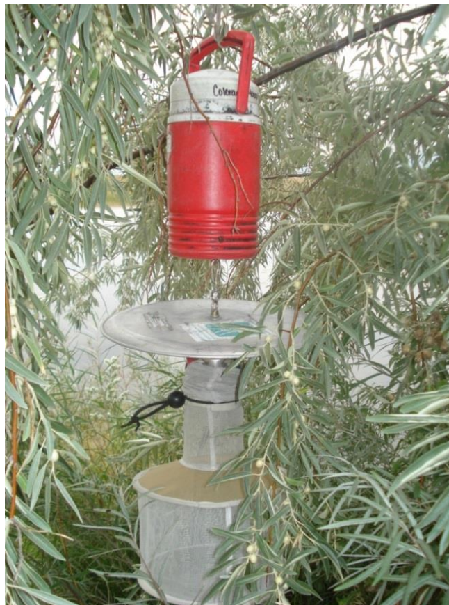
CDC light trap used to capture adult mosquitoes.
