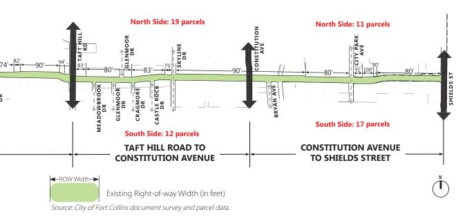
FIGURE 11: Existing Cross Section Index
