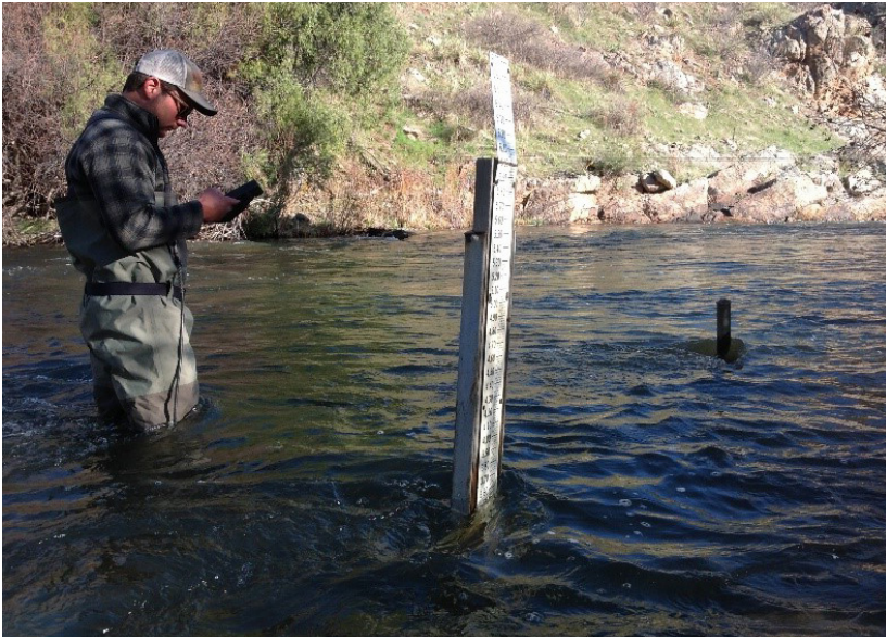
Casey Barby, Watershed Technician, collects water quality indicator data on the North Fork Cache la Poudre River in early spring using a multi-parameter water quality sonde.
