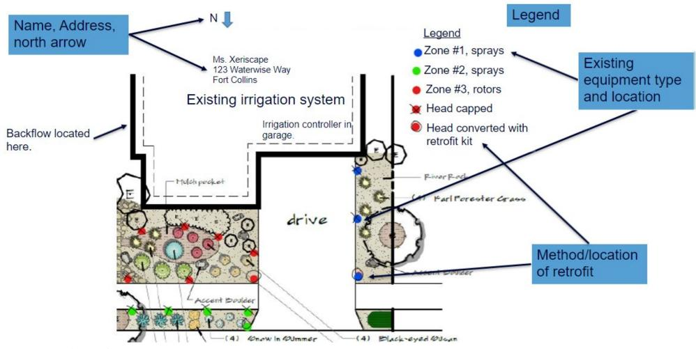
Figure 3 - Irrigation Plan Example
