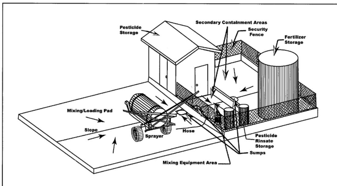
**Figure PHF-1.** Example Combined Pesticide and Fertilizer Storage and Mixing Area. Figure courtesy of *Designing Facilities for Pesticides and Fertilizer Containment*, Midwest Planning Service, Agricultural Engineering, Iowa State University 1991.
