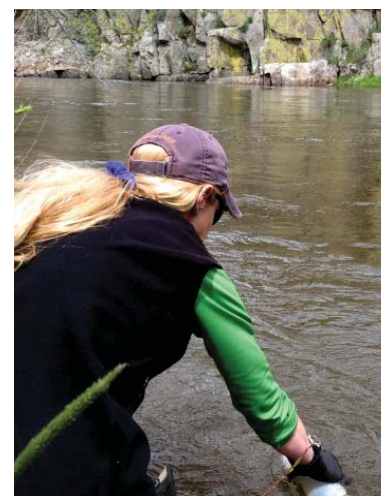
Kendra Arbesman collects a grab sample from below the City of Fort Collins raw water intake (PNF).
