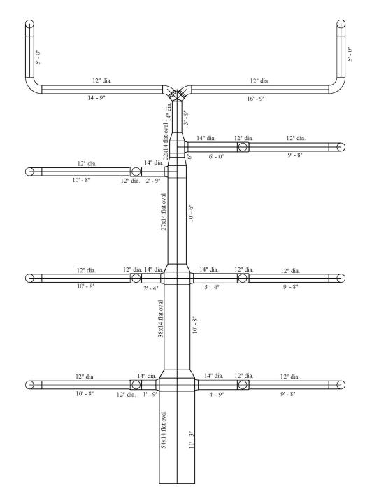
Sample layout converted to multiple runs of round spiral duct
