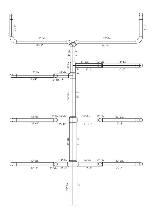
Sample layout converted to flat oval and round spiral duct
