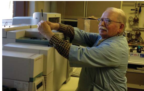
Dr. Keith Elmund injects an extracted geosmin sample into a Gas Chromatography Mass Spectrometer to quantify geosmin concentrations at PBR and PNF. These data provide early warning of potential taste and odor issues in the UCLP drinking water supply.
