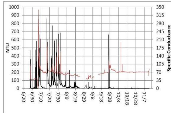
**Figure 6.** Turbidity (black solid line) and conductivity (red solid line) record from early warning system sonde located approximately four miles above the Fort Collins water supply intake facility.
