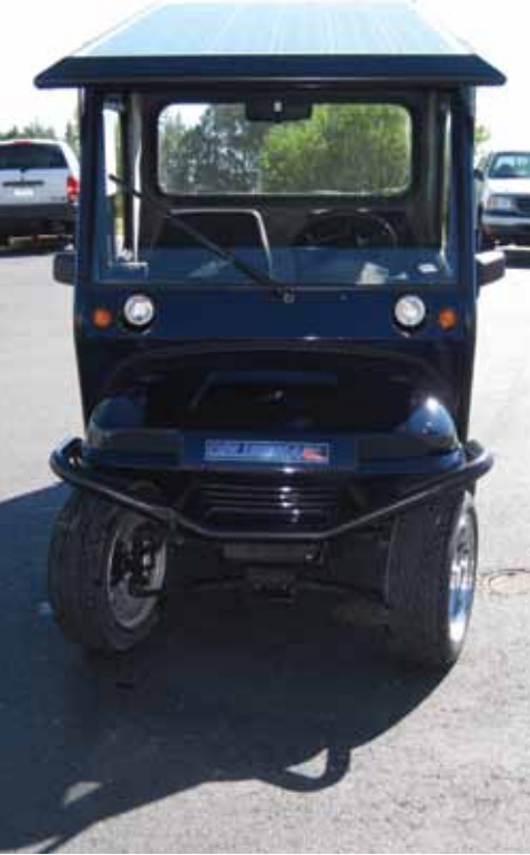
Retrofit with solar panels.
