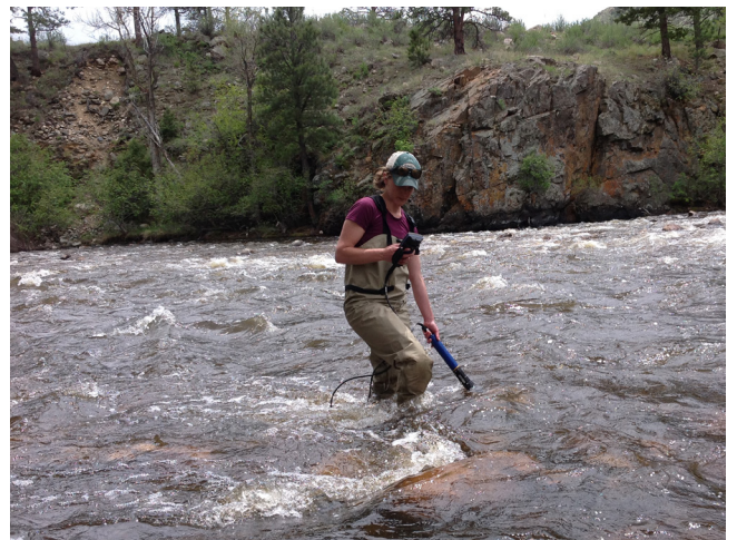
Abby Eurich, Watershed Technician, measures water quality field parameters on the Cache la Poudre River.
