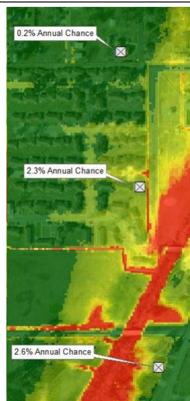
Example of flooding probability for three structures in any given year (Percent Annual Chance) The red to green color ramp shows areas of higher
