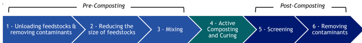
Figure 10: Typical Composting Process Flow Diagram
