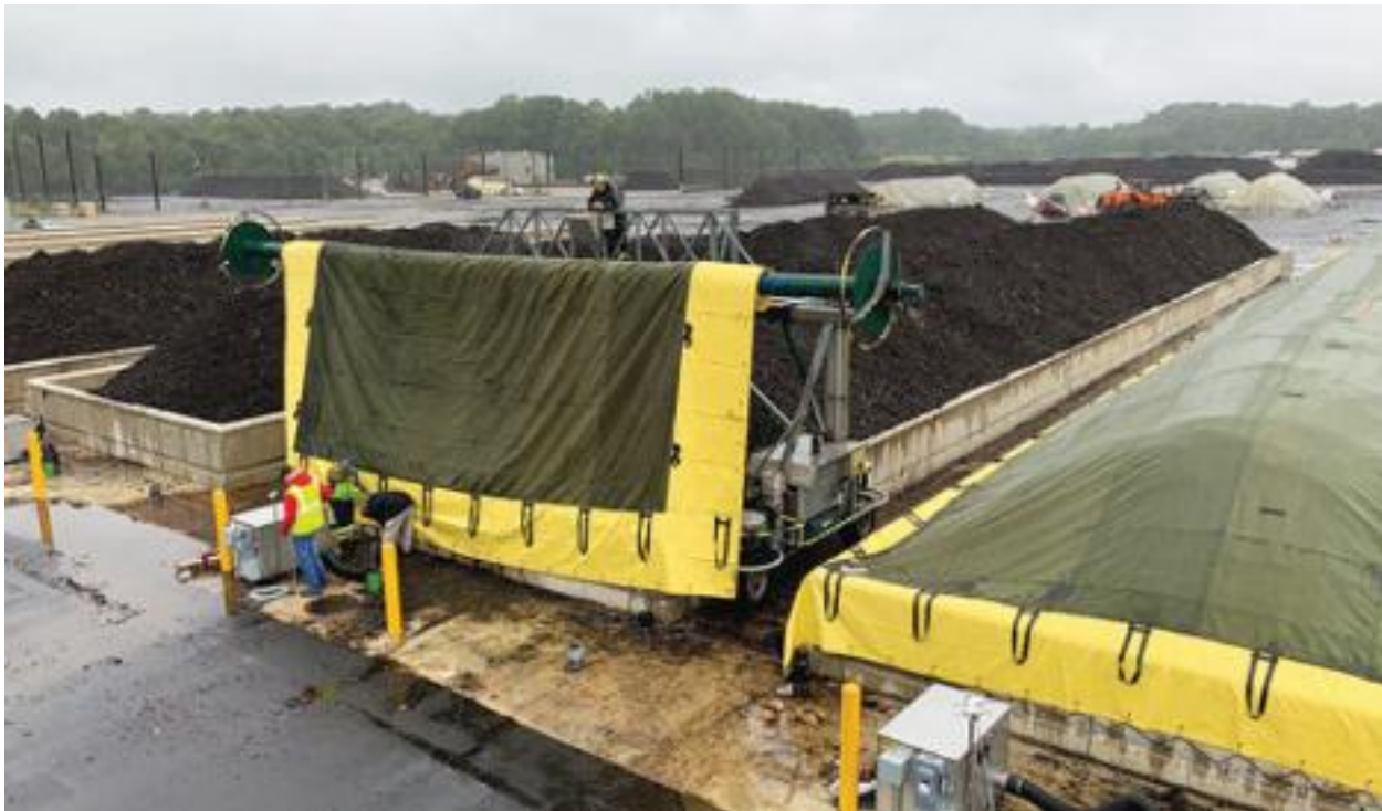
Figure 18: Sustainable Generation (SG) Example of a 65,000 TPY ASP Curbside Food Scrap and Yard Trimming Facility
