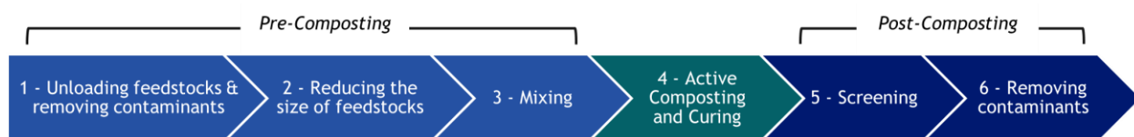
Figure 15: Aerated Static Pile (ASP) System Stages
