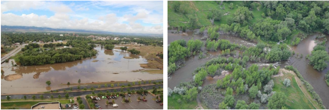
Figure 4.5: Floodplain connectivity is critical for river health, and it also reduces risk to infrastructure. During extreme high flow events, where floodplain-river connectivity is poor and development in the riparian zone is extensive, there is greater risk of flood damage to infrastructure. The photograph at left shows a connected floodplain at a former golf course (currently the Woodward site and Homestead Natural Area). Near the bottom left of the photograph, however, the intersection of Lemay Avenue and Mulberry Street limits floodplain connectivity and floodwaters threatened to over top Lemay Avenue. In contrast (right), at the ELC, the riparian zone is managed for natural habitats and the topography allows for the river to be connected to the immediate zone next to the river, resulting in a resilient situation
