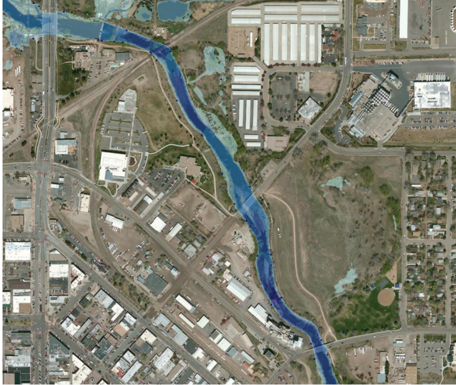
Figure 4.4a: The five-year water surface extent between College Ave. and Lincoln St. (reach 10) shows an entrenched channel with limited floodplain connectivity due to natural bedrock and constructed berms.
