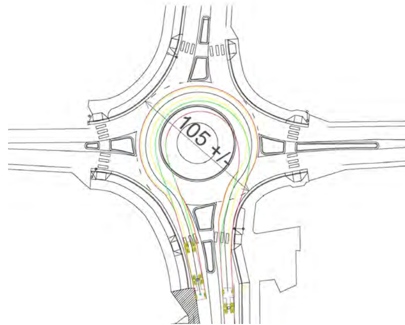
A 105' diameter roundabout is needed to accommodate a WB-40, a small delivery truck
