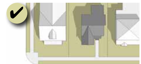
Figure 187: Locate a new building to maximize passive solar potential. This example illustrates a building (top) imposing on its neighbor's solar access.
