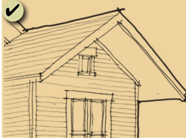
Figure 167: Provide overhanging roof eaves that appear similar in scale to those seen in the historic context.
