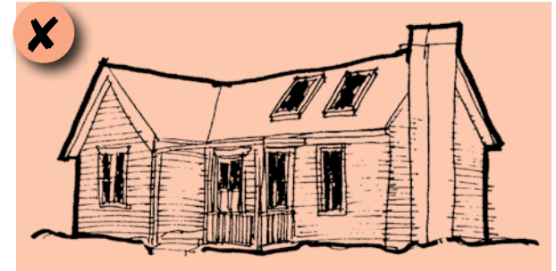
Figure 113: Do not install a dormer or skylight on a front-facing roof plane.
