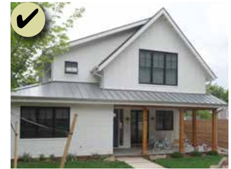
Figure 129: Design a building to be compatible with the context. A gable roof form and front porch are appropriate features; however, the porch should be raised similar to others in the context.
