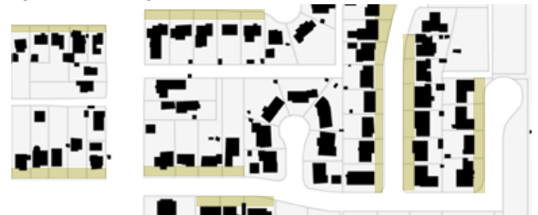
Figure 50: Building Figure Ground Map of Character Area 6. Uniform front yard setbacks occur along a block face (highlighted in green).
