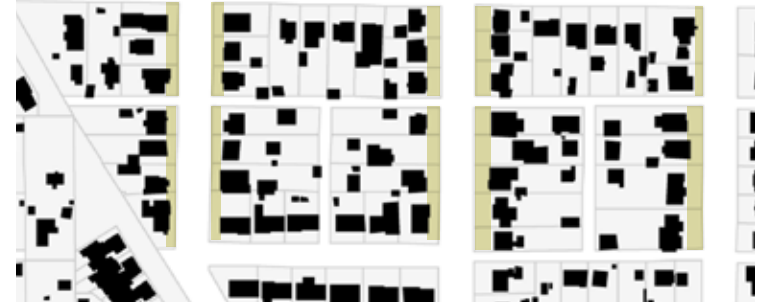
Figure 43: Building Figure Ground Map of Character Area 5. Uniform front yard setbacks occur along a block face (highlighted in green).
