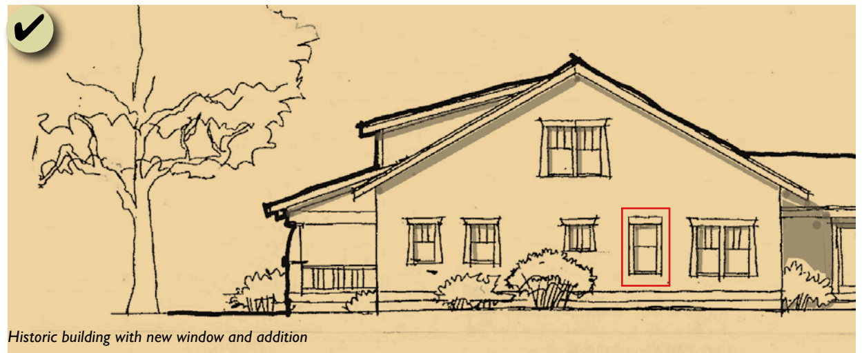
Figure 92: Design a new window opening to match historic window proportions on the same façade. The image above illustrates the historic building. The image below shows an appropriate location for a new window in the historic building.
