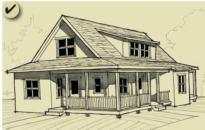
Figure 176: Locate a new dormer to the rear and/or the side (set back from the front façade) to help preserve the existing roof form and historic building materials. Also, the dormer should be located below the ridge line.
