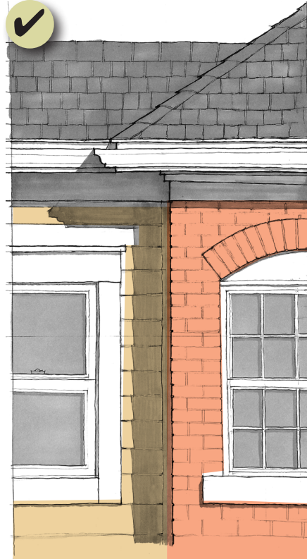
Figure 163: Wood siding is an appropriate material. Note this addition uses a narrow wood lap to differentiate it from the existing building.
