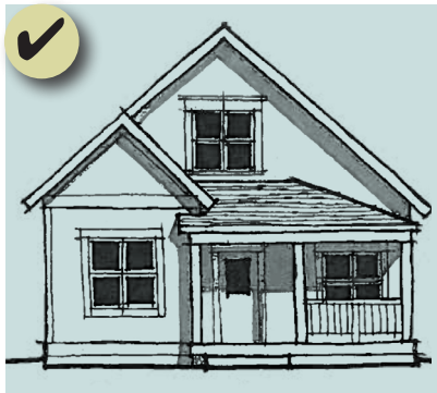
Figure 131: Design a building to be compatible with the context. Providing a gable roof and one-story elements that step down to the street are appropriate features on this building.
