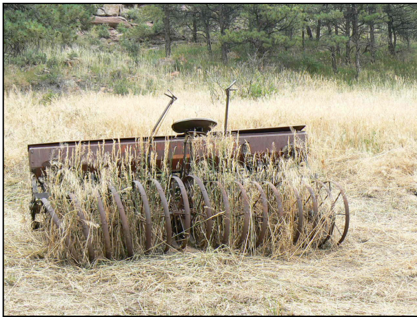
Figure 73. Press wheel drill for planting grain seeds like alfalfa, oats, or wheat.
