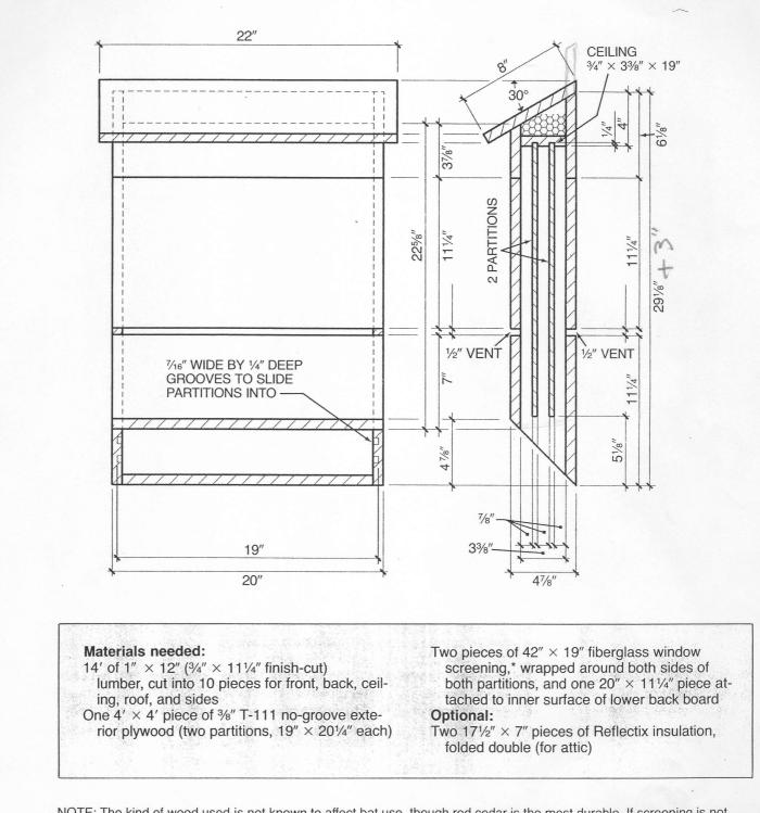
NOTE: The kind of wood used is not known to affect bat use, though red cedar is the most durable. If screening is not used, vertical grooves should be cut narrower to %" to ensure a tighter fit. At least one wood surface in each chamber, plus the inner surface of the lower back board, must then be roughened or slightly grooved (horizontally) to provide a surface for bats to cling to.
