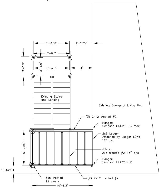
Existing Stairs with Landing: The intention is that the stairs as a complete unit including the landing will be disconnected from the existing upper landing, and moved approximately 2' west, to be approximately 4' from the exterior garage wall. The stairs are to be attached to the new larger landing.
