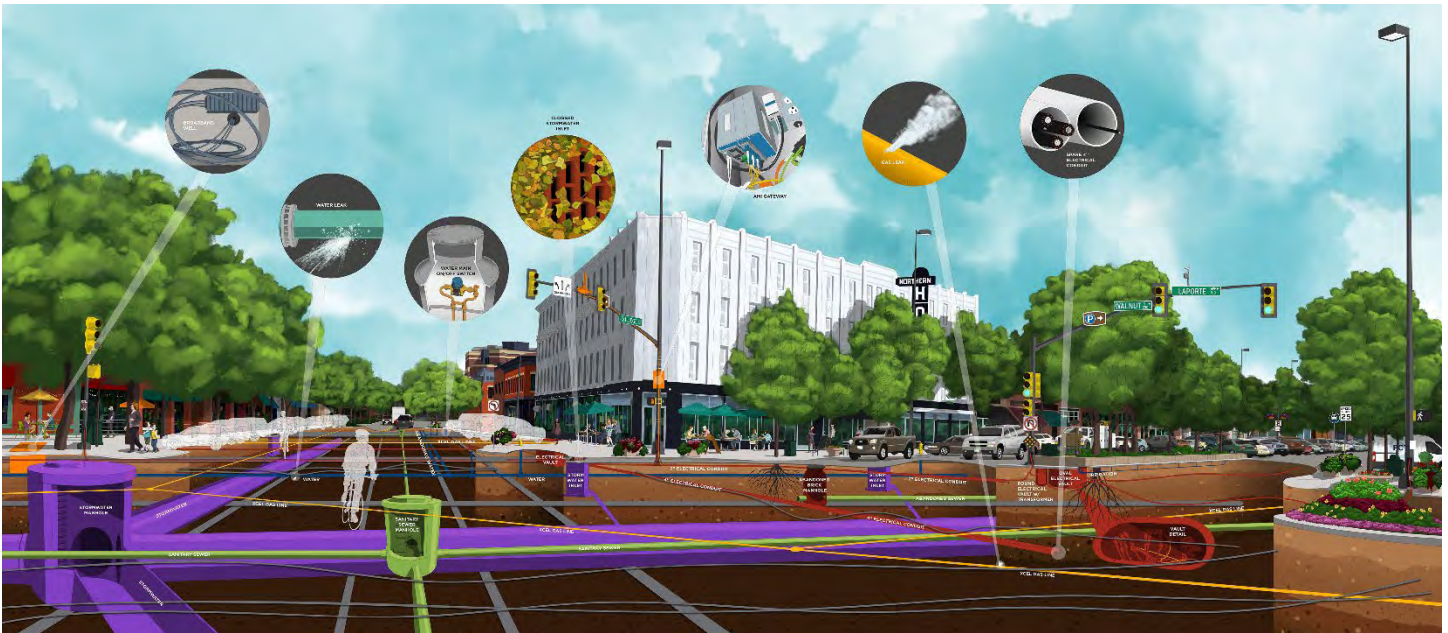
Figure 5: Example of existing dry and wet utilities within an intersection
