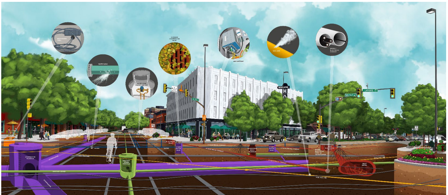
Figure 7: Example of existing dry and wet utilities within an intersection
