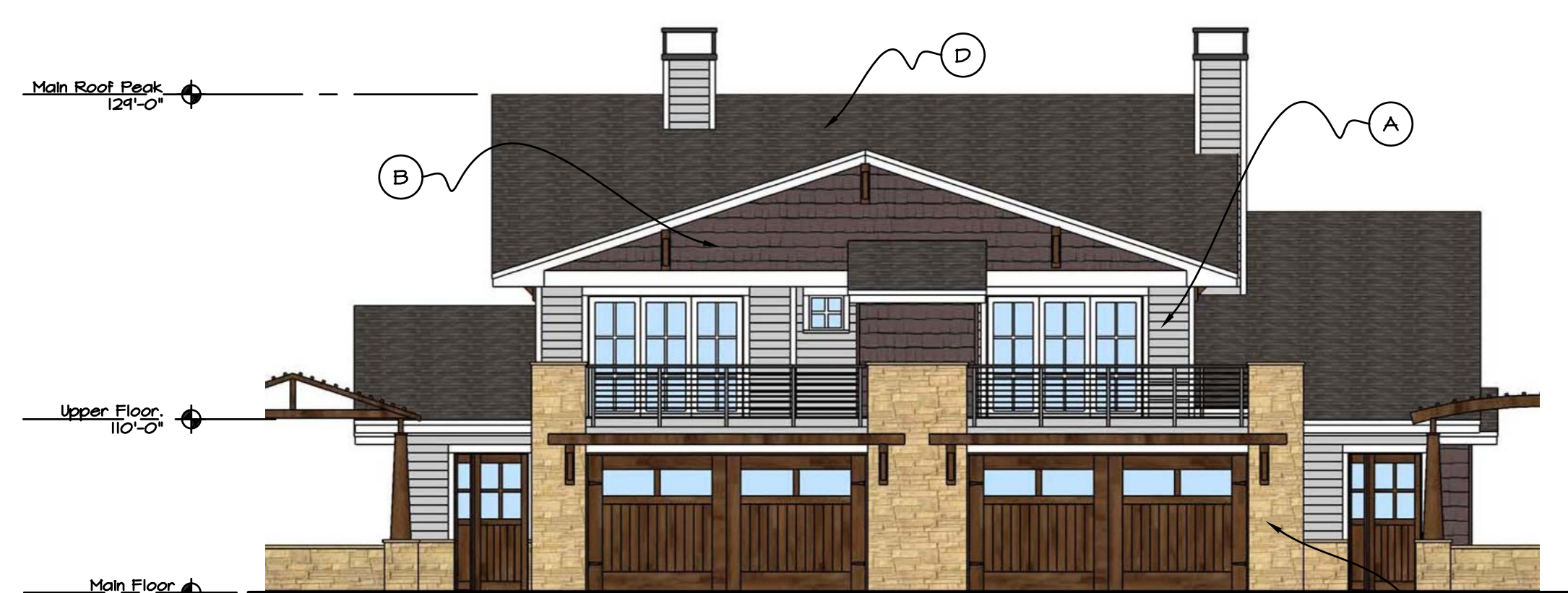
6 BUILDING TYPE 2 - Front Elevation SCALE: 1/8" = 1'-0" BUILDING TYPE 2: Duplex with Unit A and Unit B - for Lots 1, 2, 7-14, 17 or 18
