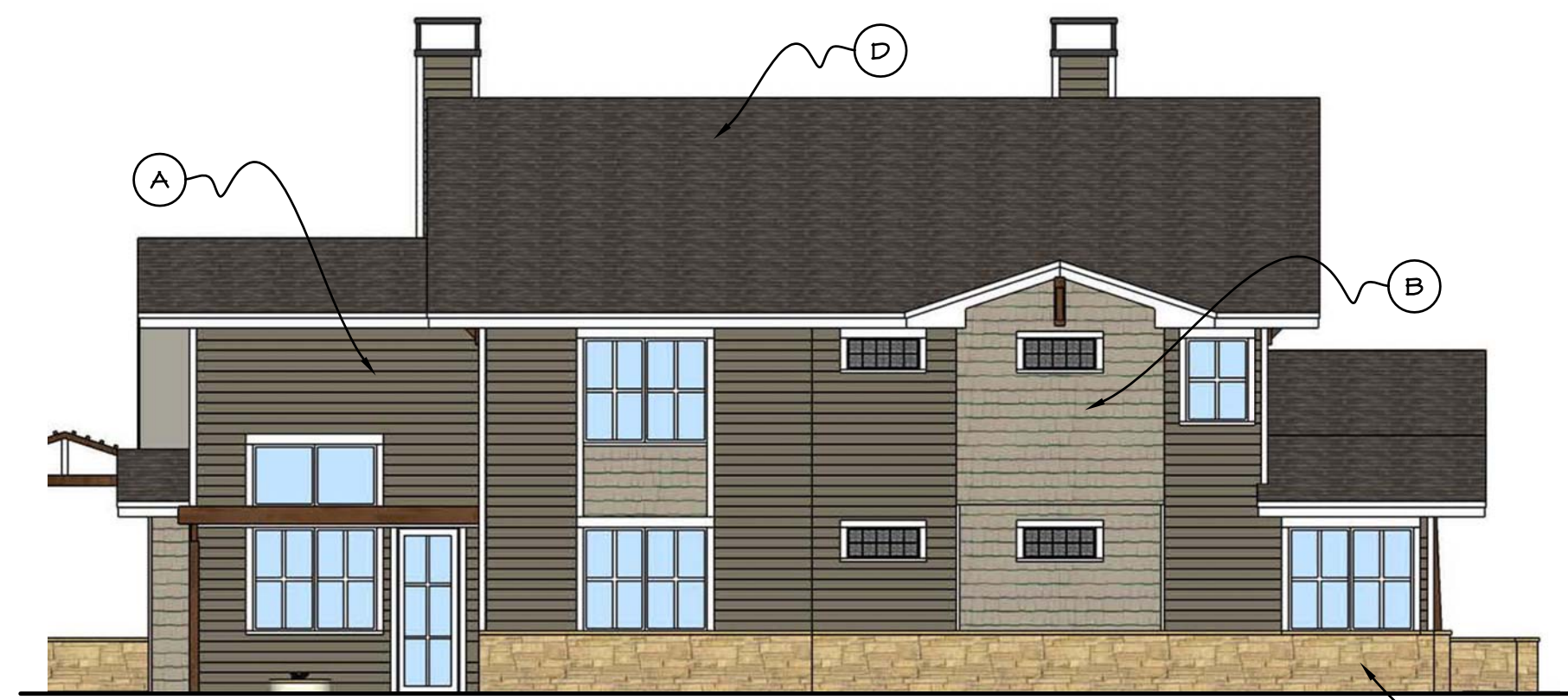
4 BUILDING TYPE 1 - Rear Elevation SCALE: 1/8" = 1'-0" BUILDING TYPE 1: Duplex with Unit A and Unit B - for Lots 1, 2, 7-14, 17 or 18
