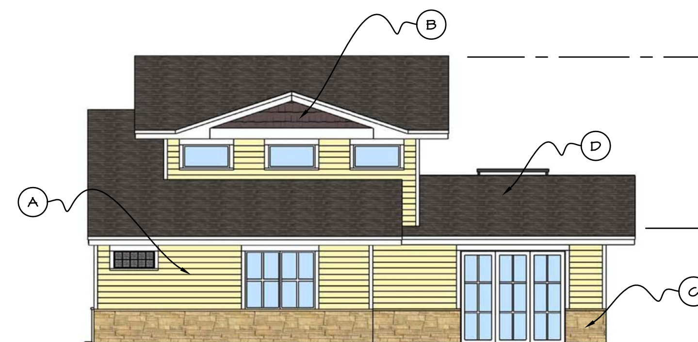
7 BUILDING TYPE 6 - Rear Elevation SCALE: 1/8" = 1'-0" BUILDING TYPE 6: Single Unit C - for Lots 3 & 4
