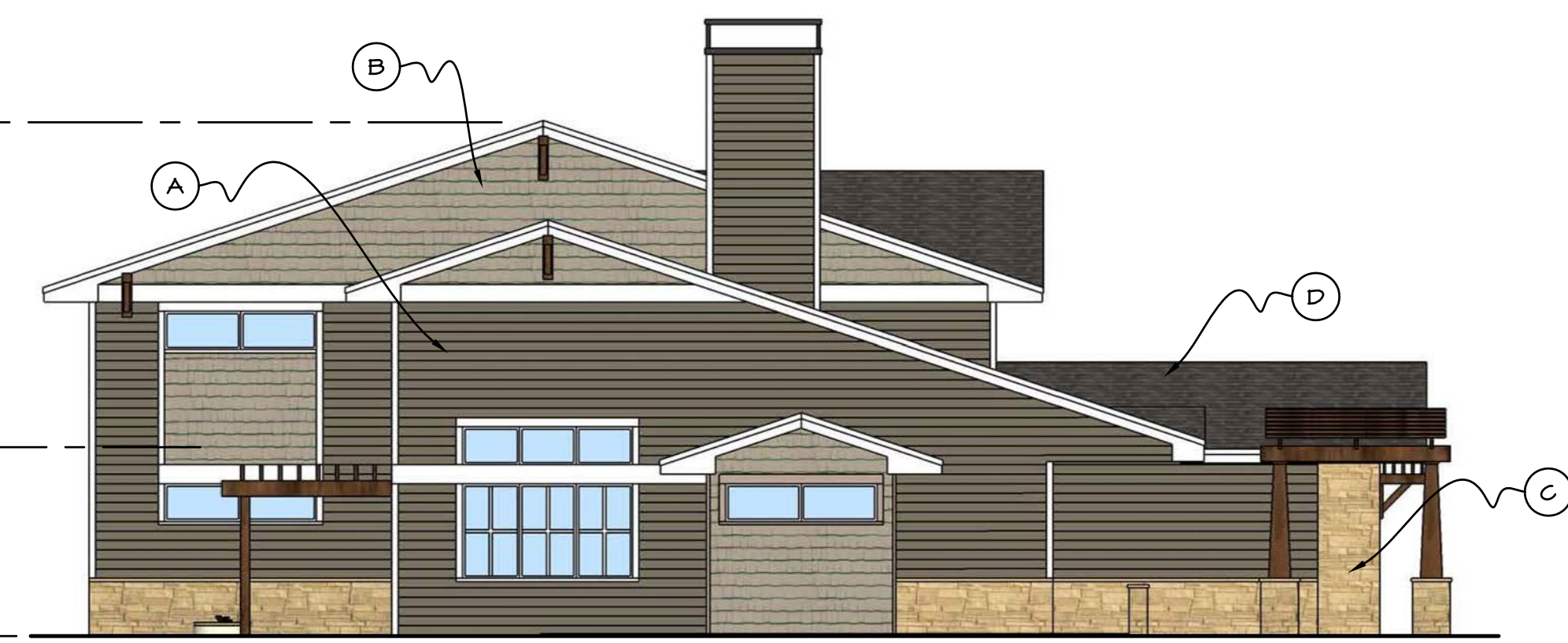
⑧ BUILDING TYPE 4 - Left Side Elevation SCALE: 1/8" = 1'-0" BUILDING TYPE 4: Duplex with Unit B2 and Unit B2 - for Lots 5, 6, 15 or 16
