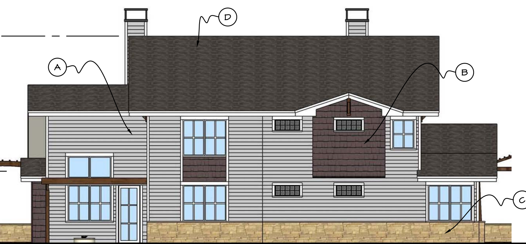
8 BUILDING TYPE 2 - Rear Elevation SCALE: 1/8" = 1'-0" BUILDING TYPE 2: Duplex with Unit A and Unit B - for Lots 1, 2, 7-14, 17 or 18
