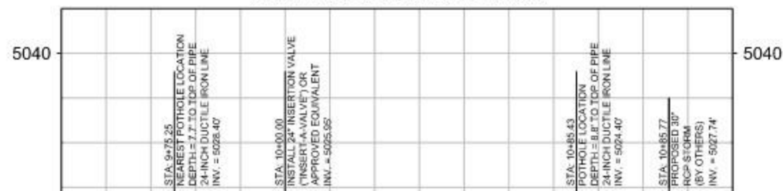
Trilby 24-IN D.I. Water (WEST) PROFILE SCALE: (H) 1" = 20' (V) 1" = 2' START STA: 9+50.00, END STA: 11+00.00
