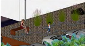
H. Dry stream bed (or path) along north side of church building, infiltrates stormwater from the roof (at least 10' from foundation)
