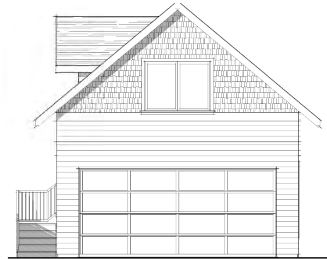
5 SD9 SD GARAGE EAST ELEVATION SCALE: 3/16" = 1'-0"
