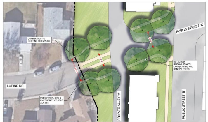
Major Amendment plan with alternative connection for peds, bikes, and emergency access
