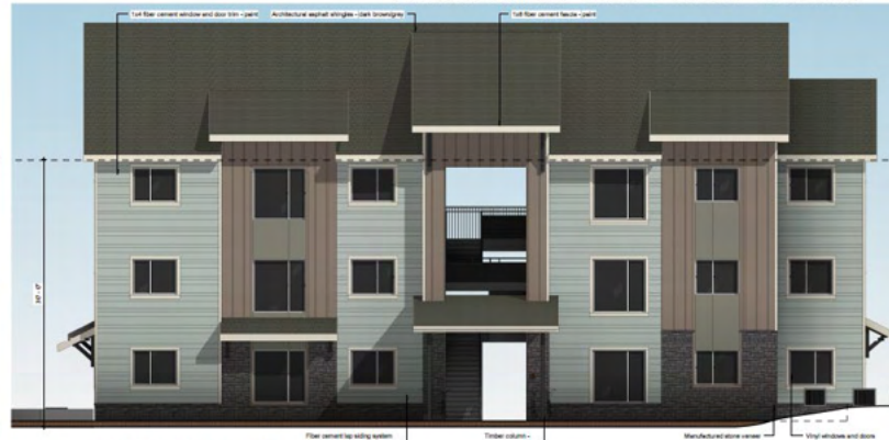
Building C Front Elevation
