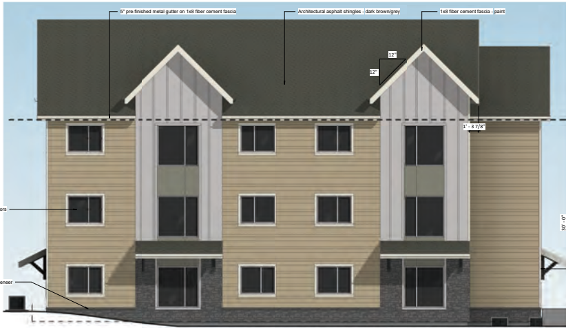
Bldg. A Back Elevation 3 VDP4 SCALE: 3/32" = 1'-0"
