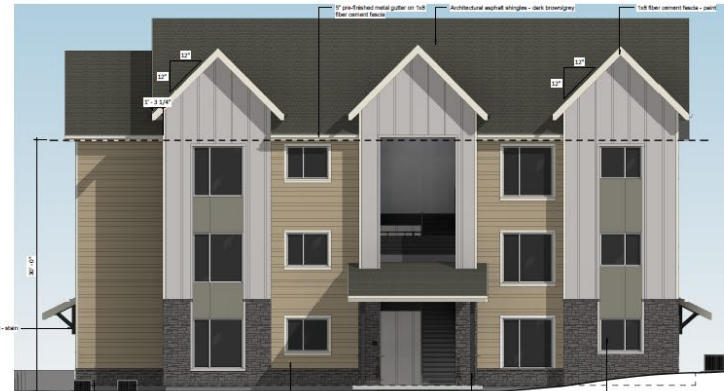
Bldg. A Front Elevation
