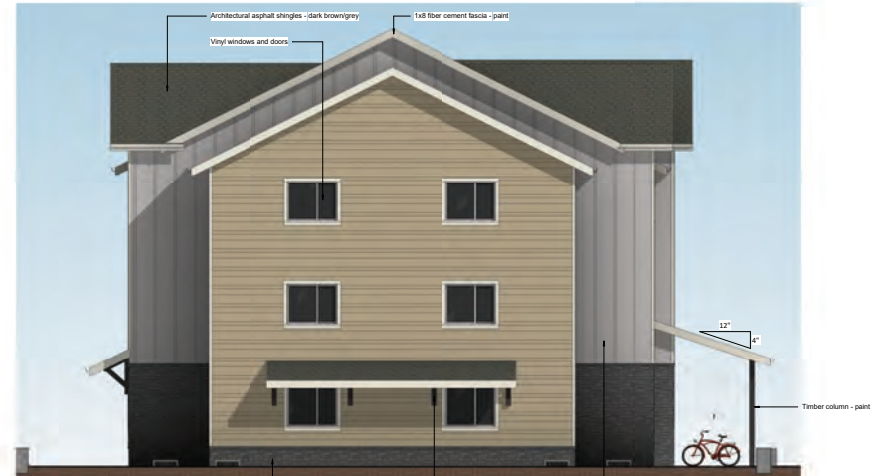
Bldg. A Side 2 Elevation 4 VDP4 SCALE: 3/32" = 1'-0"
