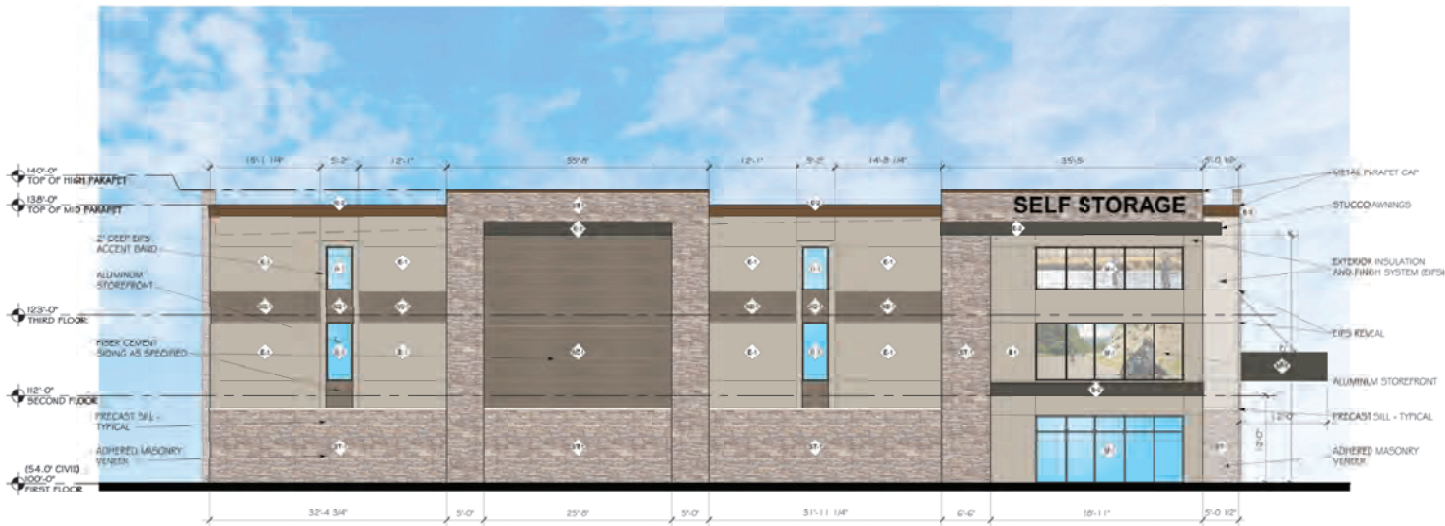
1 THREE STORY BUILDING "A" - NORTH EAST ELEVATION SCALE: 1/8" = 1'-0"
