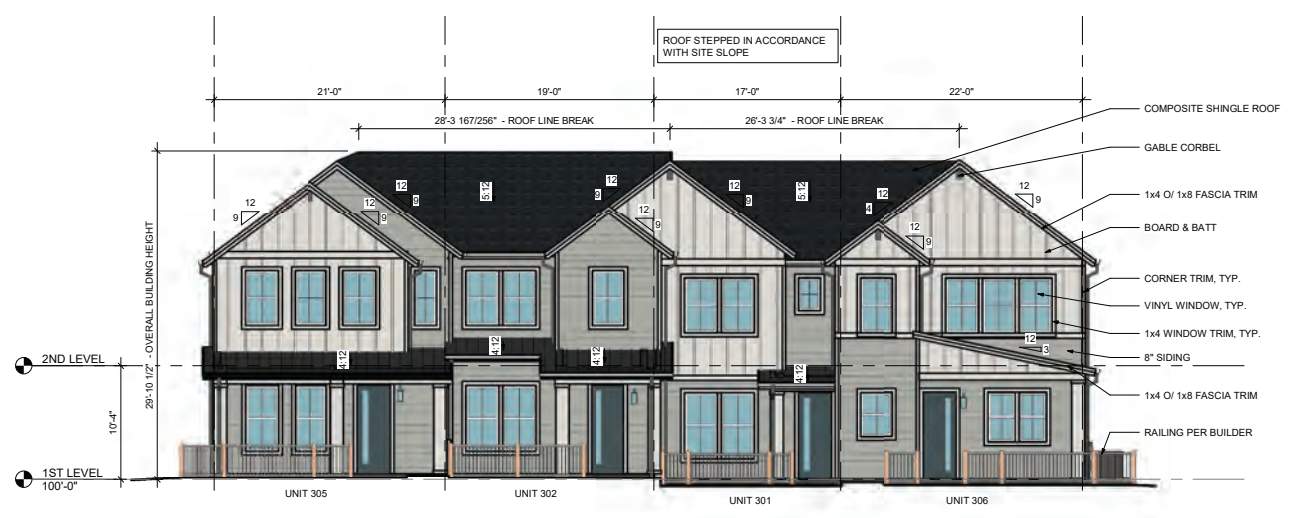
1 4-PLEX - CONTEMPORARY FARMHOUSE - FRONT ELEVATION 1/8" = 1'-0"
