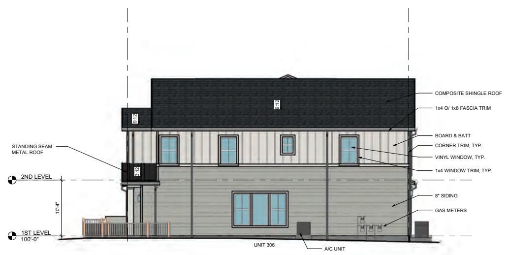
2 4-PLEX - CONTEMPORARY FARMHOUSE - RIGHT ELEVATION 1/8" = 1'-0"
