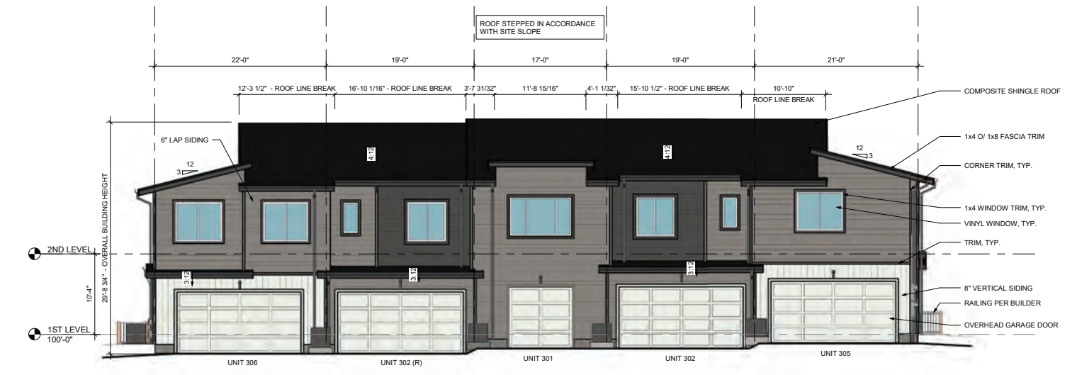
3 5-PLEX - COLORADO MODERN - REAR ELEVATION 1/8" = 1'-0"
