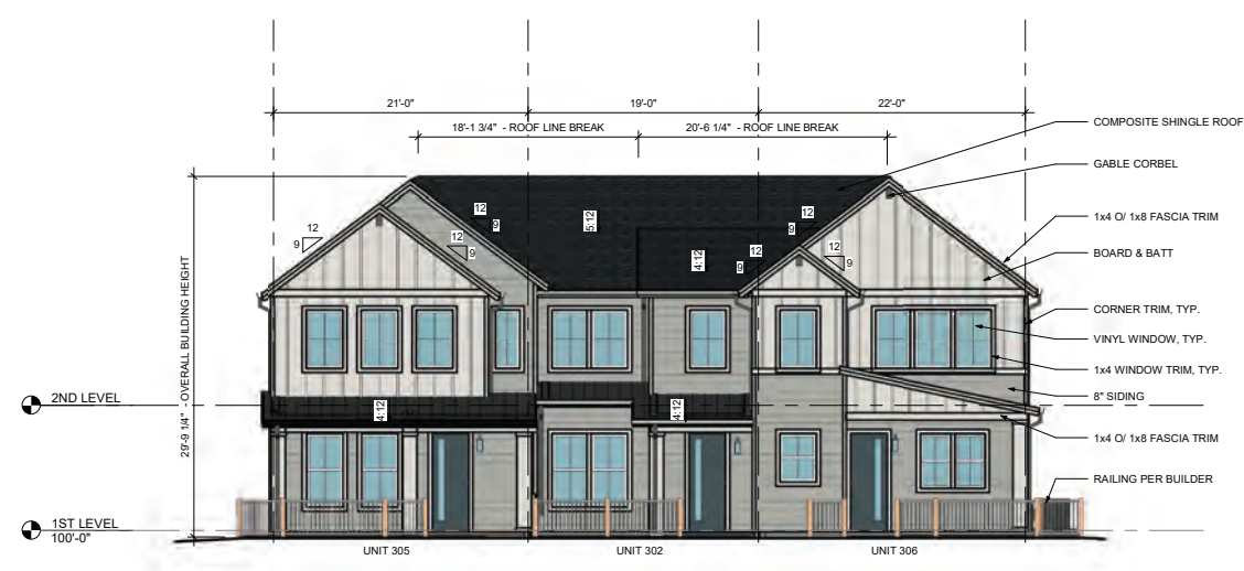
1 3-PLEX - CONTEMPORARY FARMHOUSE - FRONT ELEVATION 1/8" = 1'-0"
