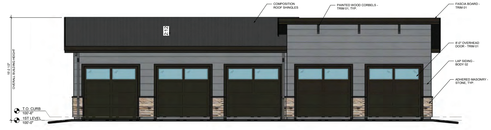
4 GARAGE A - FRONT ELEVATION 1/4" = 1'-0"
