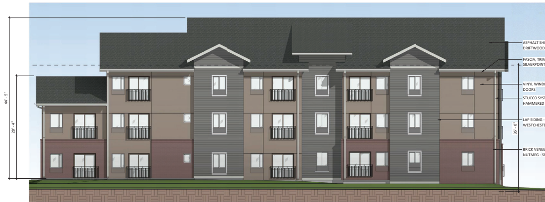
1 BUILDING 1 - EAST ELEVATION A-02 SCALE: 1/8" = 1'-0"
