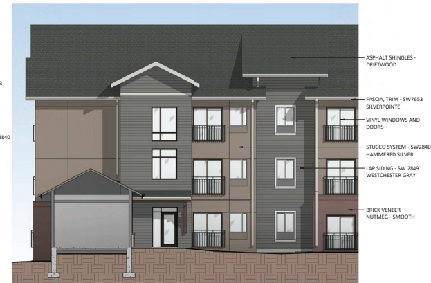
2 BUILDING 1 - WEST PLAZA ELEVATION A-02 SCALE: 1/8" = 1'-0"
