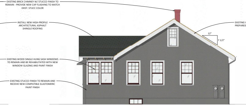
BUILDING 3 - EAST ELEVATION
