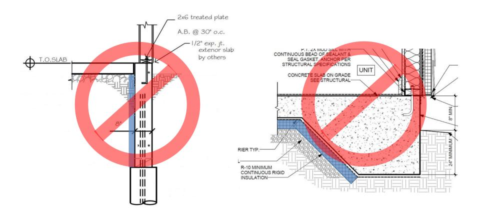
Drawings directly above: Insulation does not meet minimum code requirement.
