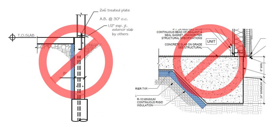
Drawings directly above: Insulation does not meet minimum code requirement.
