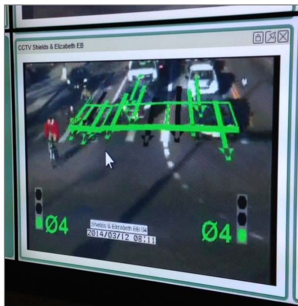
FIGURE 27: EXAMPLE SCREEN DISPLAY SHOWING DETECTION ZONES PROVIDED WITH VIDEO DETECTION EQUIPMENT
