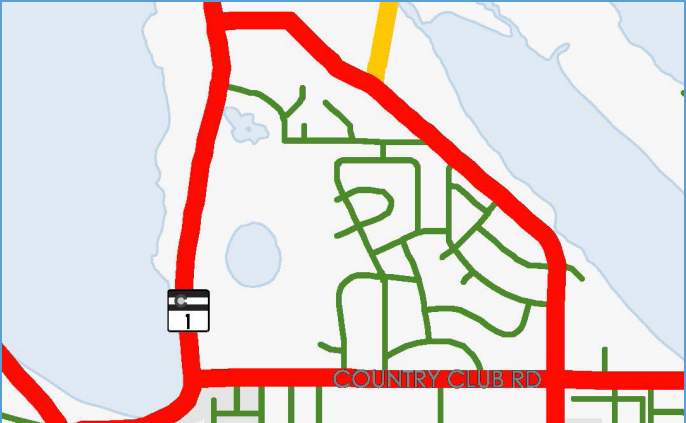
Thin green lines denote low stress streets. Red and yellow lines denote higher stress streets.
