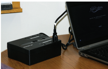
An uninterruptible power supply (UPS) is useful for protecting sensitive equipment, such as computers or network servers and minimizes immediate losses.
