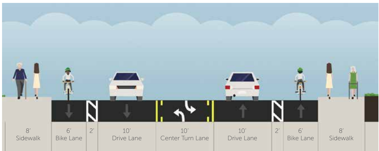
This Streetmix cross-section represents the conceptual striping recommendation for West Mulberry between Taft Hill Road and City Park Avenue (Segment 1), including one vehicle travel lane each direction, a new center turn-lane, and buffered bike lanes. Future sidewalk widening may also occur.
