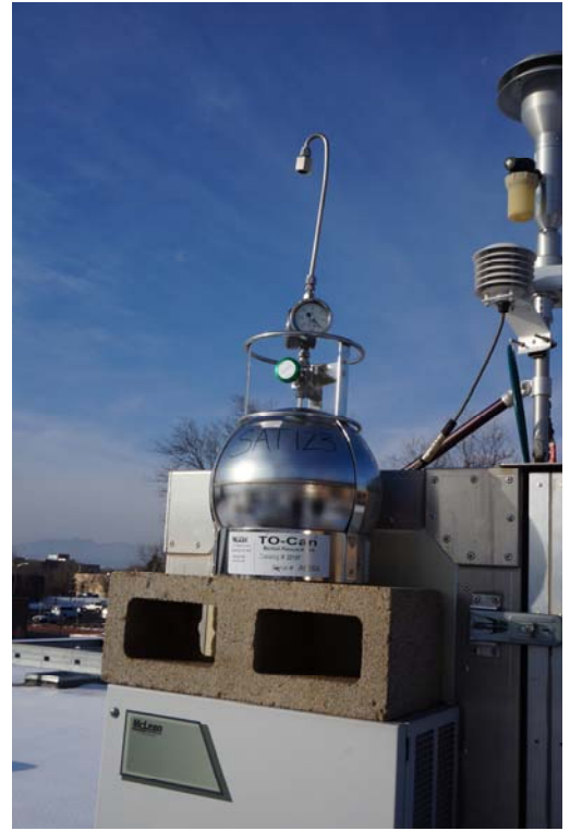
Figure 2-3. VOC sample canisters located at the City Park (CPFC) site (left) and the Mason Street (MSFC) site (right).
