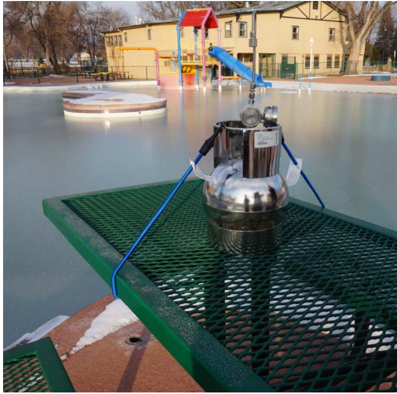
Figure 2-3. VOC sample canisters located at the City Park (CPFC) site (left) and the Mason Street (MSFC) site (right).
