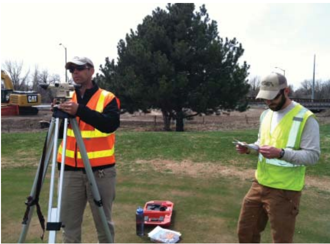
Surveying in monitoring wells at site along the river (Photo by Dave Myers)
