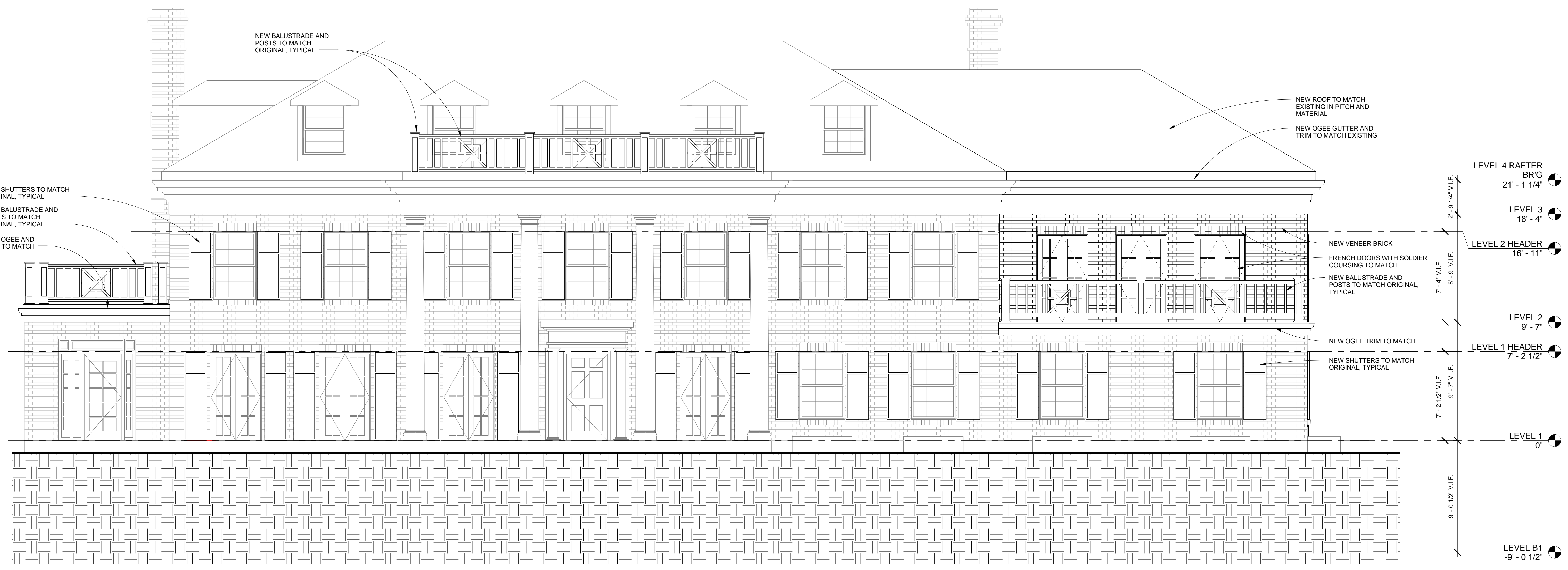
1 NORTH ELEVATION 1/4" = 1'-0" NOTE: HALFTONED OR SCREENED LINEWEIGHTS ARE INTENDED TO INDICATE EXISTING COMPONENTS OF THE BUILDING.
