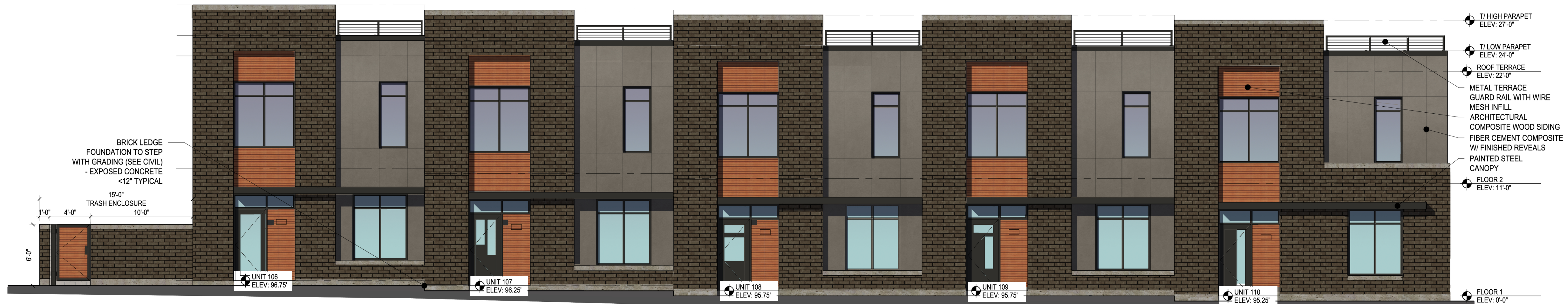
2 WEST ELEVATION - FACING ADJACENT APT. BLDG. SCALE: 1/4"=1'-0"
