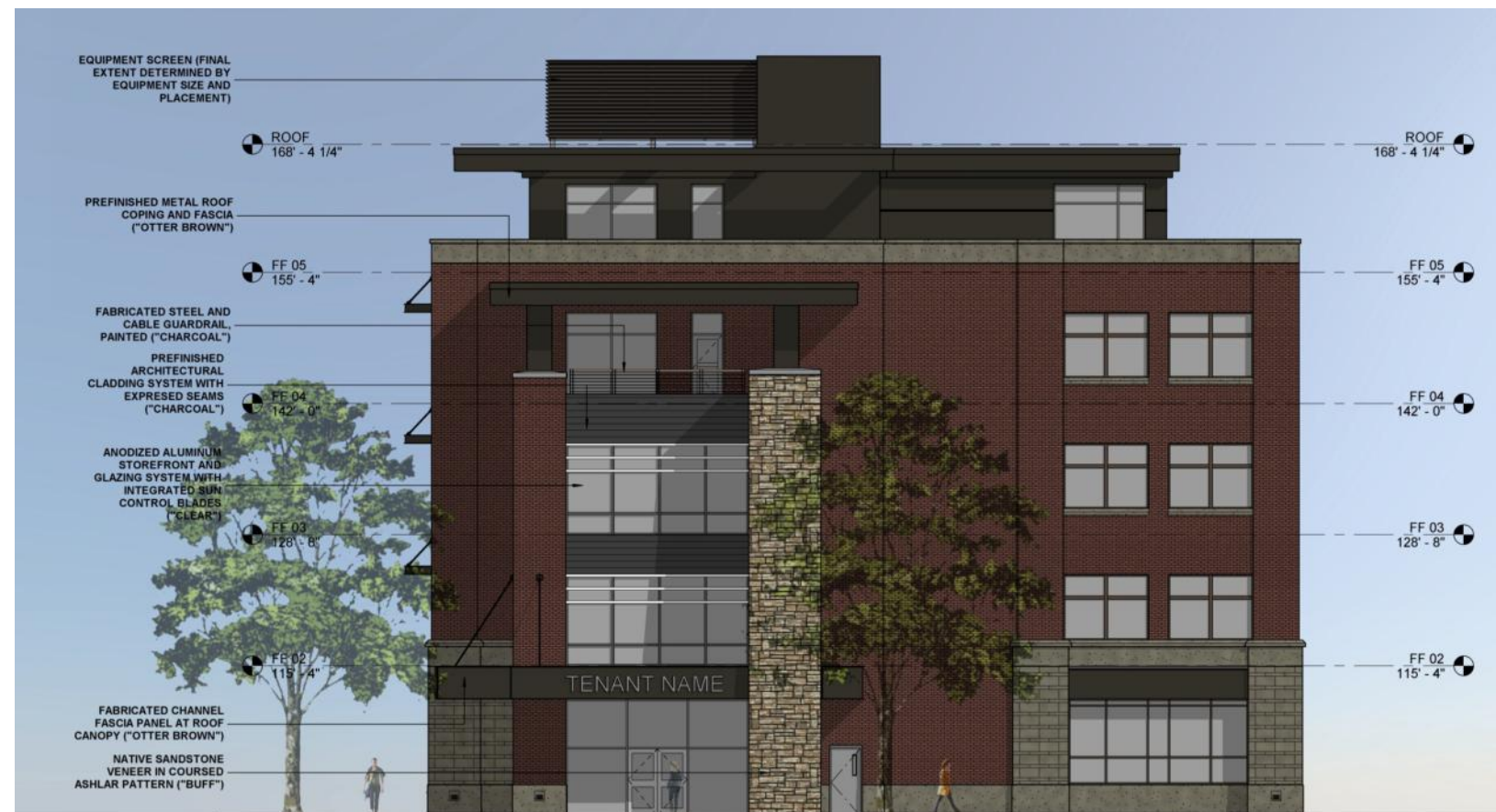
EAST (MELDRUM STREET) ELEVATION
