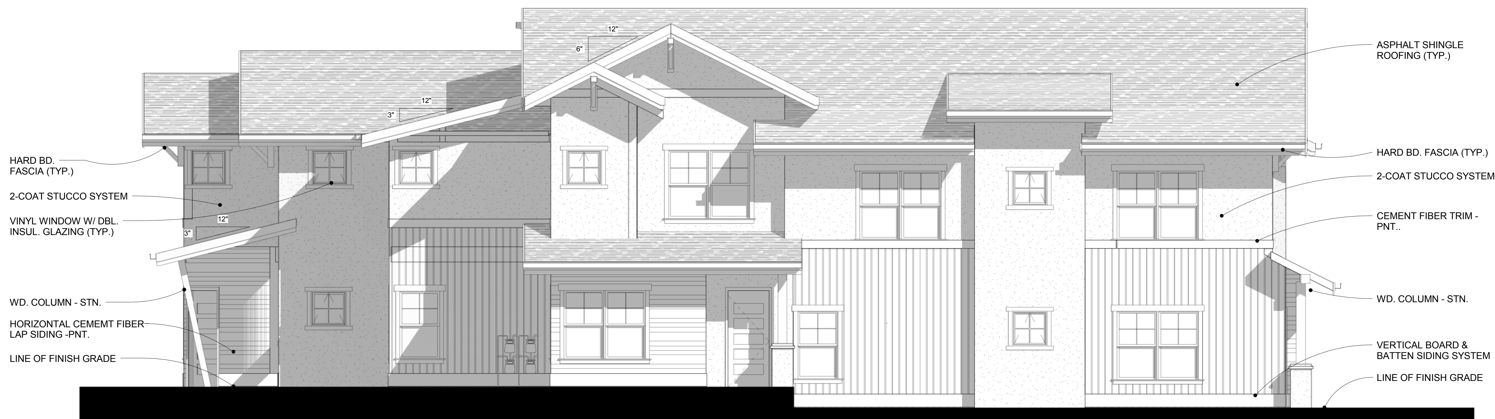
4 Building South Elevation 1/4" = 1'-0"
