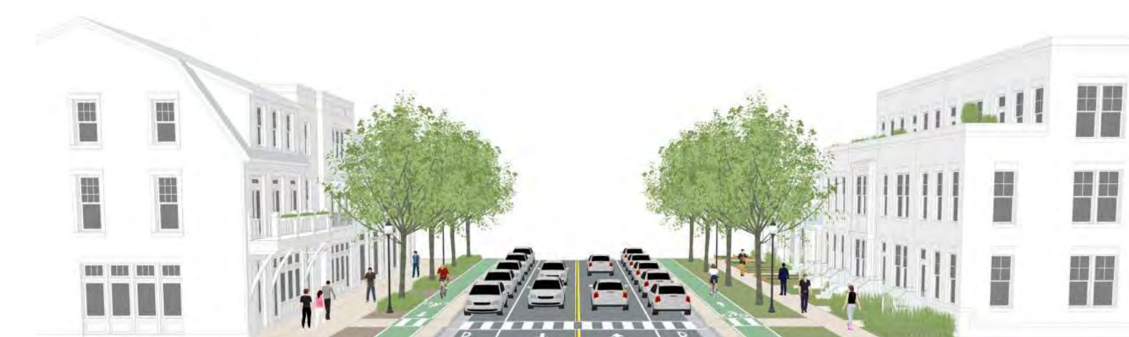
4 Minor Collector Right-of-way: 80' Roadway: 54'
