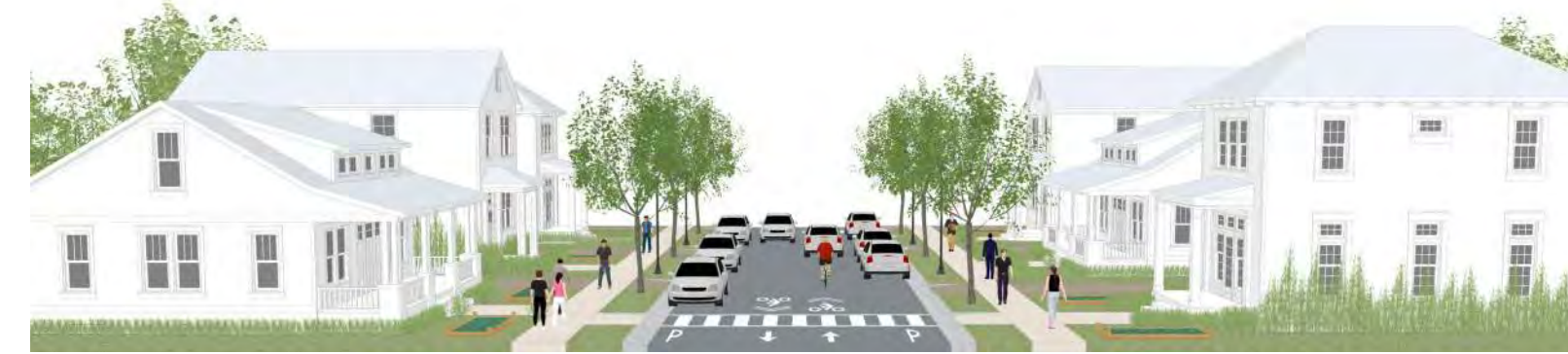
6 Residential Local (without alley) Right-of-way: 53' Roadway: 30'
