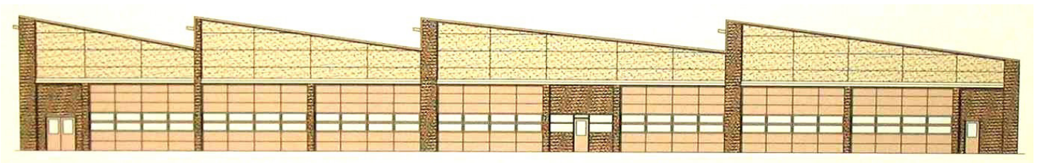
The sawtooth roof design, with high south-facing windows, provides daylighting throughout the building.
