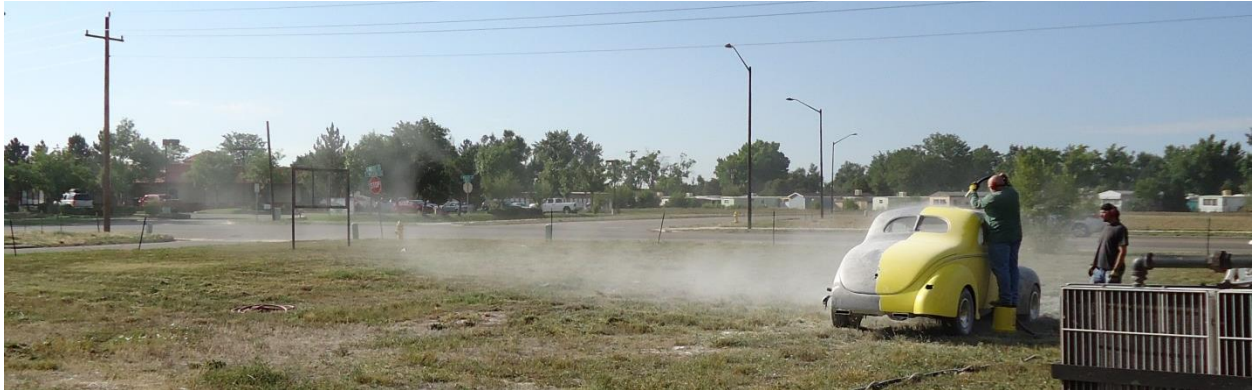
Above: This photo illustrates abrasive blasting without dust mitigation in place.
