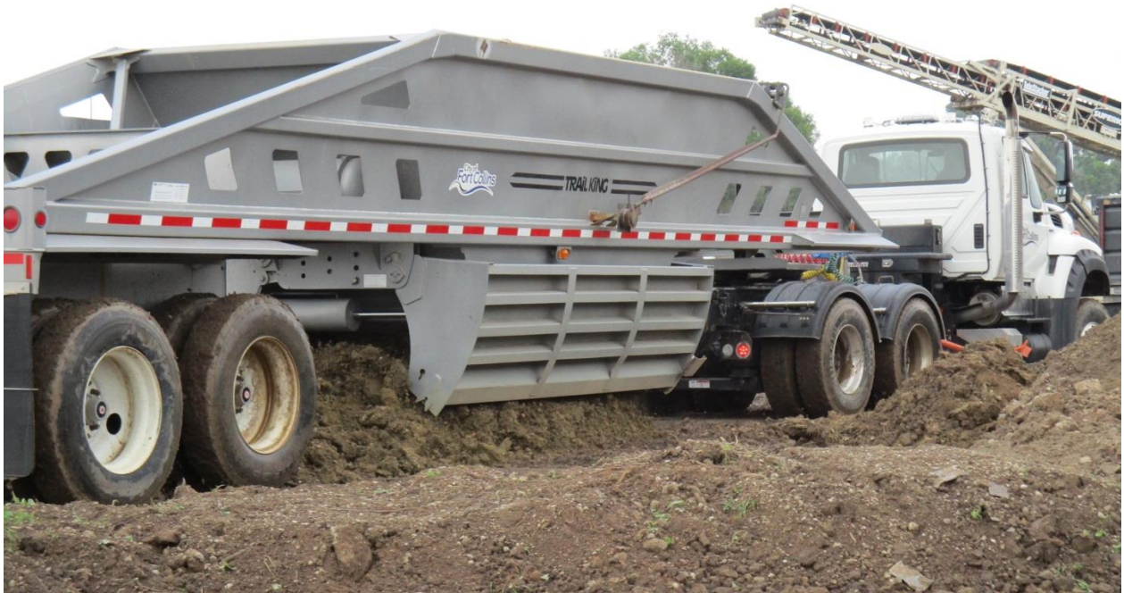
Above: This figure illustrates minimizing drop heights, a required best management practice for bulk materials transport.
