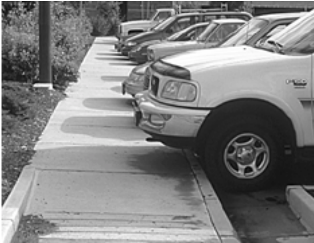
6 feet — the bare minimum allowed by the standards. Can work for secondary or utilitarian walkways.
