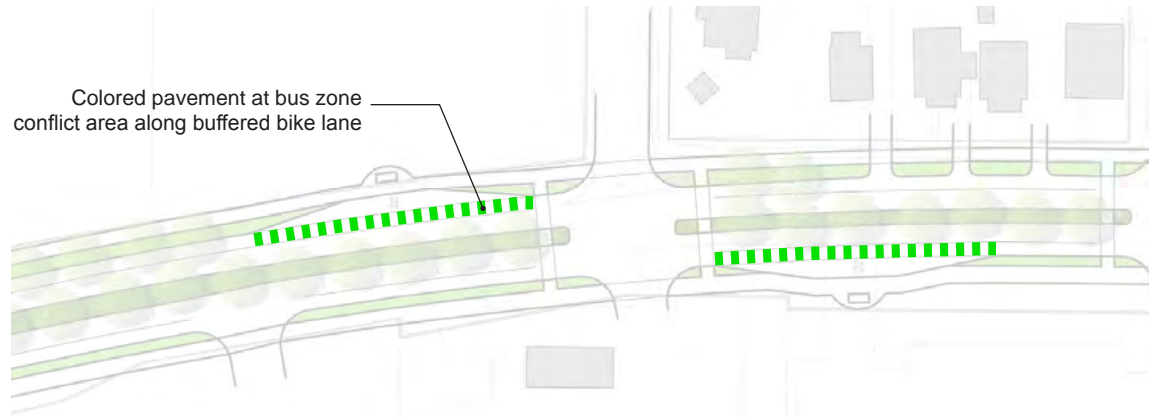
The use of colored pavement mark the potential conflict area for buses and bicyclists along Lincoln Avenue.
