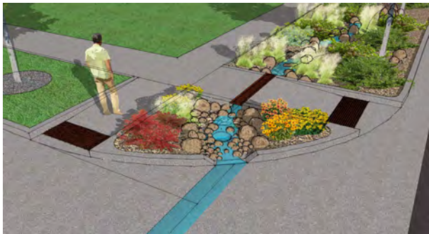
A bioswale at a pedestrian crossing
